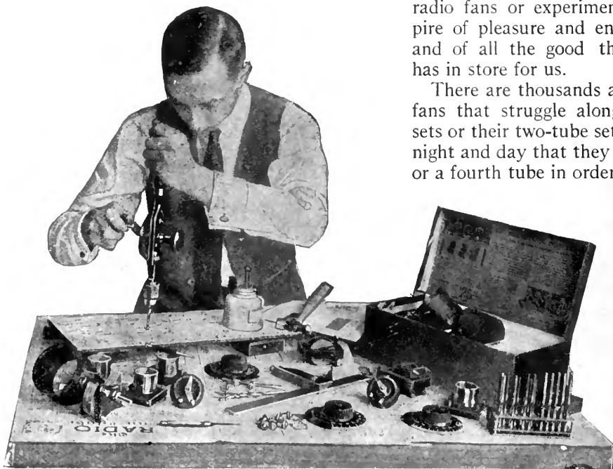
THE SET UNDER WAY Mr. Stark is shown drilling the panel, preparatory to assembling a receiver such as he describes in this article
