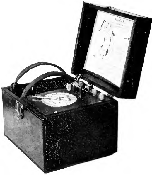
A CRYSTAL RECEIVER One of the first to be made specially for broadcast reception
